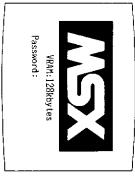
If you have forgotten the password, you can start the system by holding down the **GRAPH** and the **STOP** keys and pressing the RESET button until the display changes.
